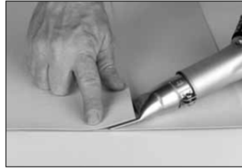
Tack Weld (for detailing only)
